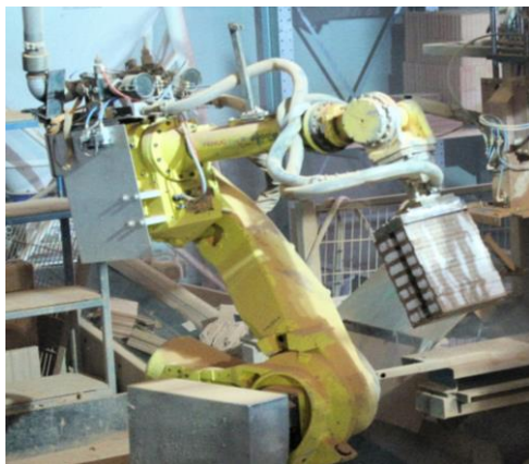
Fig. 12. The robotic masonry fabrication technique gives a precise positioning of bricks with the stretch display of the curving walls
