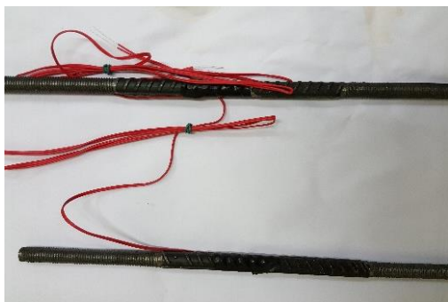
b) Strain Gauges in Steel Shear Bolts
