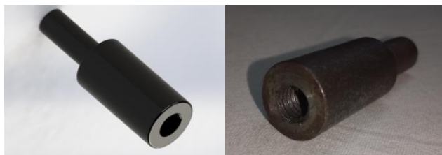
Fig.24 T-section Design and Actual Part
