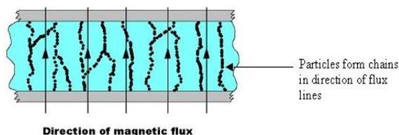
**Fig. 2:** MR Fluid in presence of Magnetic Field
