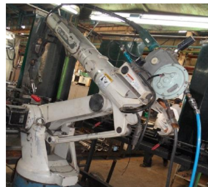
Fig.1 Welding Robot (OTC Daihen DR -4000)
