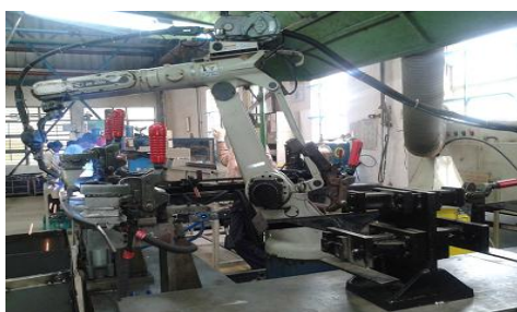
Fig.4 Robot working on two fixture positions
