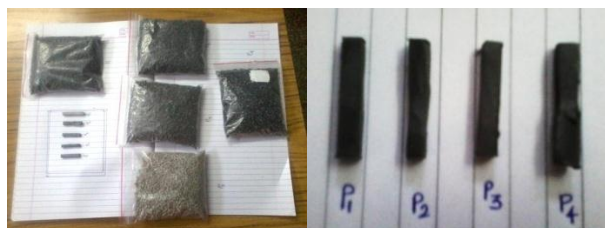
Fig 1: Granules of PEEK composite and injection molded pins
