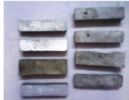
Figure 9 Dimensions of prepared specimen-40*40*170
