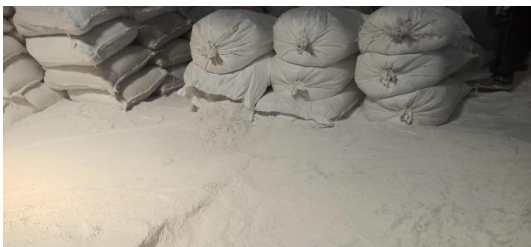
Fig. 2 Raw-Mix bags burst due to excess pressure
