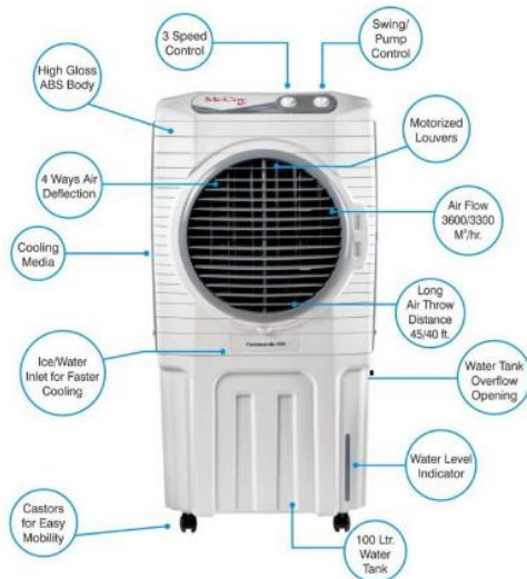
Fig. 2: Parts of a typical air cooler
