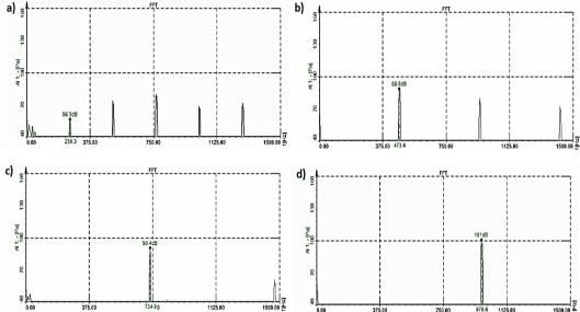
**Figure 7.** FFT for frequency levels [a] 250Hz, [b] 500Hz, [c] 750Hz, [d] 1000Hz and constant sound pressure source100 dB with composition 40% Coco Peat and 60% of Recycled Rubber
