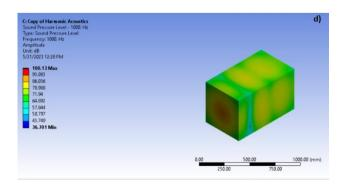
**Figure 8.** FFT Analysis on Ansys for Frequency [a] 250Hz, [b] 500Hz, [c] 750Hz, [d] 1000Hz at constant sound pressure source 100dB with composition 40% Coco Peat and 60% of Recycled Rubber
