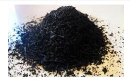
Figure 2. Secondary material recycled rubber.
