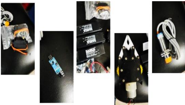
Fig. 1 Components used in the creation of Robotic arm, Starting from left; servo motor, IR sensor, battery gripper and metal sensor
