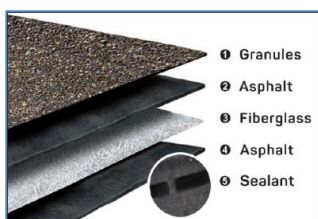
Fig.1: Roof Shingles with numbers of layers
