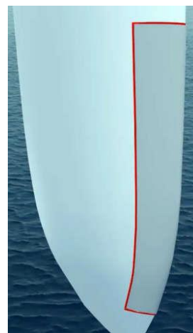
Figure9: Application of anti-corrosion coating on wind turbine blade leading edge
