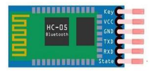
The HC-05 shown in Figure is a Bluetooth module that works according to the SPP (Serial Port Protocol) principle. This module is specially designed for wireless serial communication. This module is equipped with Bluetooth V2.0 EDR (Enhanced Data Rate) 3 Mbps modulation with a full 2.4 GHz radio transmitter and base frequency. It uses CSR Bluecore
