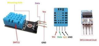
DHT11 is a temperature and humidity device. The sensor comes with an NTC sensor to measure temperature and an 8-bit microcontroller to output temperature and humidity values as serial data. The sensor is also factory calibrated so it is easy to interact with other microcontrollers. The sensor can measure temperature from 0°C to 50°C and humidity from 20% to 90% with accuracy of  $\pm$ 1°C and  $\pm$ 1%. Therefore, if you want to measure within range, this sensor will be a good choice for you.
