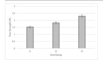
Figure 7: Tear strength variations of fabricated interlining samples.
