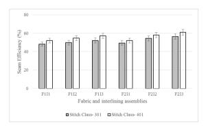
**Figure 13:** Seam efficiency comparison of developed fabric and interlining assemblies' samples.
