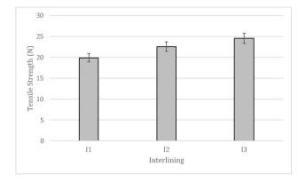
Figure 8: Tensile strength variations of fabricated interlining samples.
