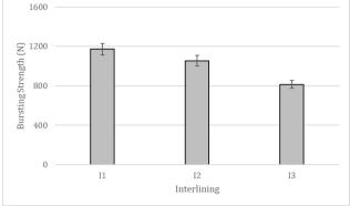
Figure 10: Bursting strength variations of fabricated interlining samples.
