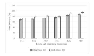
Figure 12: Seam strength comparison of developed fabric and interlining assemblies' samples.
