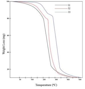
Figure 11: TGA of fabricated interlining samples.
