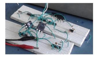
The phase detector of the digital circuitry is made with d flip flops. The clock pulse of the d flip flops of Fr must be less than the clock pulse of the d flip flop from the VCO. Fvco/N. This frequency generation is very tough and the analog circuitry gives better result than the digital circuitry. The regular clock pulse may not match with this data even the matching of this pulse is also very complicated which makes this circuit to gives lesser accurate result and introduction of noise [12].
