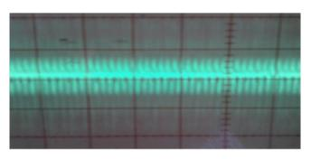
The output frequency generated in the analog circuit is very high but the noise level is under control.
