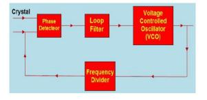
comparator, which is proportional to the phase difference between the signals applied at its two
