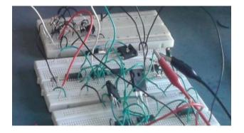
The phase detector is designed with the analog components of using clipper, integrator diodes, resistors, capacitors.
