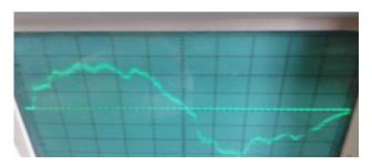
The noise level is very high in this circuit due to the mismatch of the clock pulses and the frequency generated is also very low.
