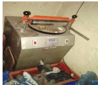
Fig.2 Semi-automatic rotti making machine with single roller and supporting plate
