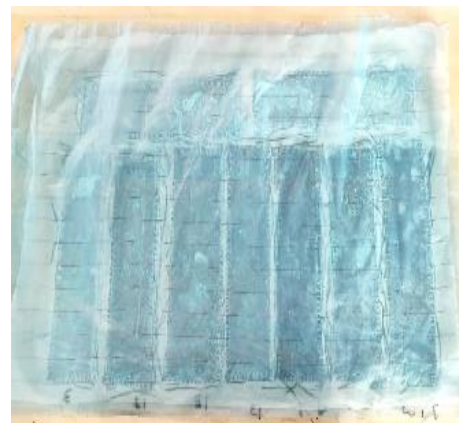
Fig: 2.1 Applying Resin and Vacuum bagged after hand lay-up
