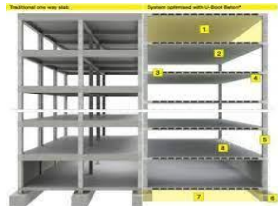
Fig.3 Comparison for Non- Voided and Voided Slab
