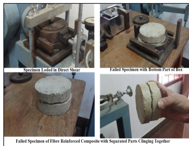
Fig.6: Direct Shear Test
