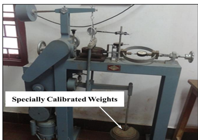
Fig.5: Conventional Direct Shear Apparatus with Modifications
