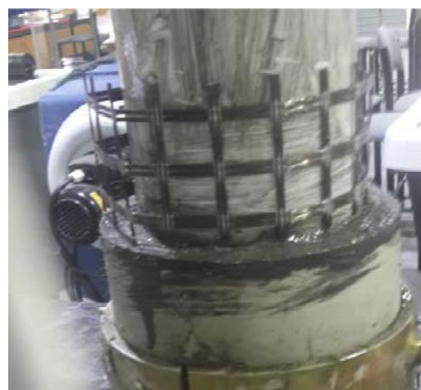
Fig.3 confinement layer casting
