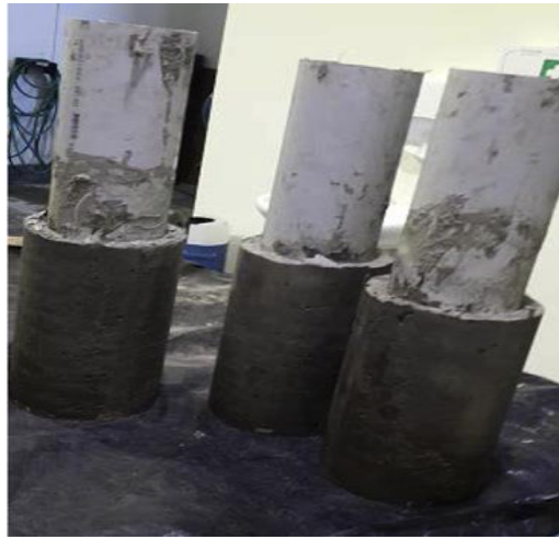
Fig.4 Removing of PVC Pipe
