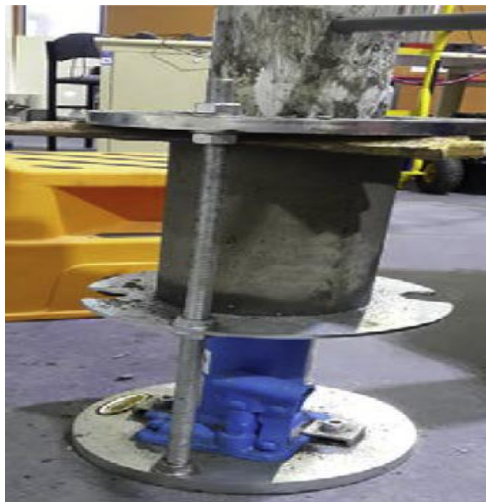
Fig.5 Removing of PVC Pipe
