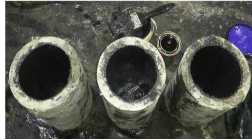
Fig.7 Lubricating the Inner Portion of Confinement Layer.
