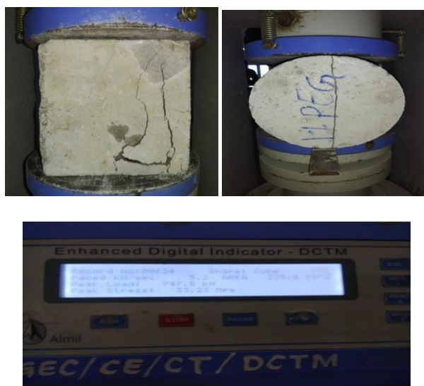
Fig. 6: Compressive and Split tensile strength test of the concrete
