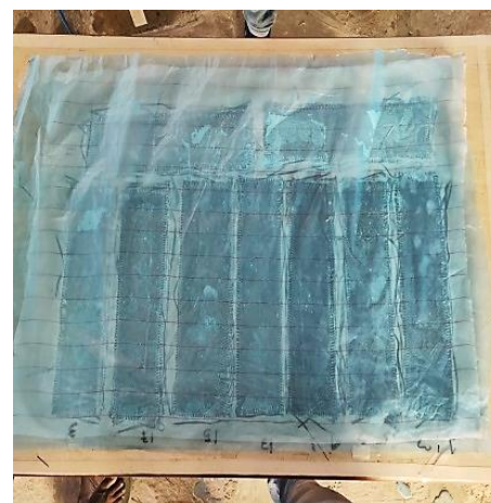
Fig: 3.1 Tailored fiber to standard and Vacuum bagged after hand lay-up
