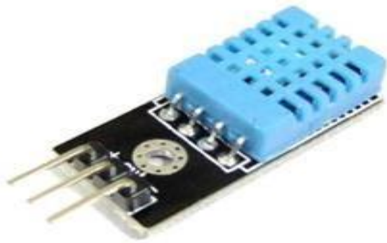
Figure 5. DHT11 Temperature and humidity sensor
