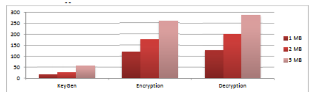
Figure 3 : Data encryption performance based on data size
