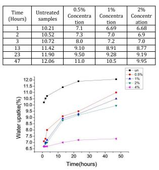
Fig.7 Water uptake of treated and untreated samples verses time (CF<sub>8</sub>)
