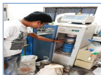
Figure 4: Compressive Strength Test Setup in CTM
