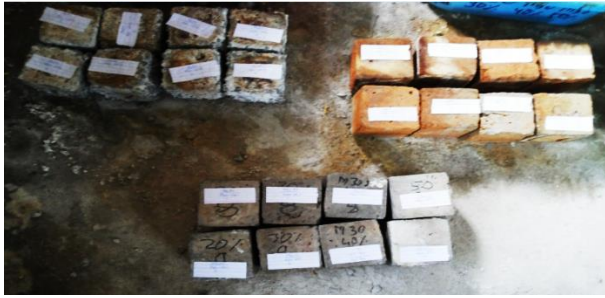
Figure 6: Concrete Cube Specimens Exposed to HCl, H_2SO_4 and Na_2SO_4 at 56 days
