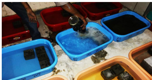
Figure 5: Concrete Specimens Absorbed in HCl, H 2 SO 4 and Na 2 SO 4
