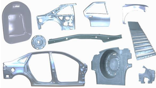
Fig. 5: Deep drawn automobile parts
