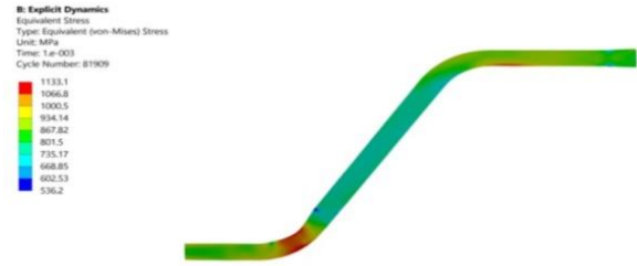
Fig. 20: Stress contour (3.5 mm thickness)
