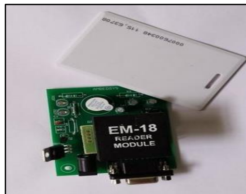
Fig.5 RFID system – Reader & Tag
