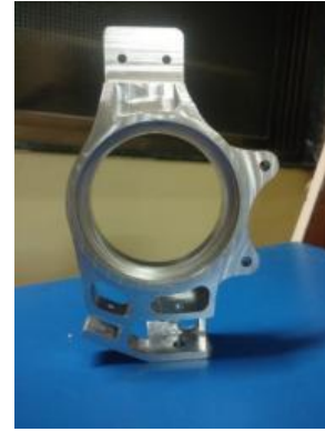
Fig 27 Finished rear upright
