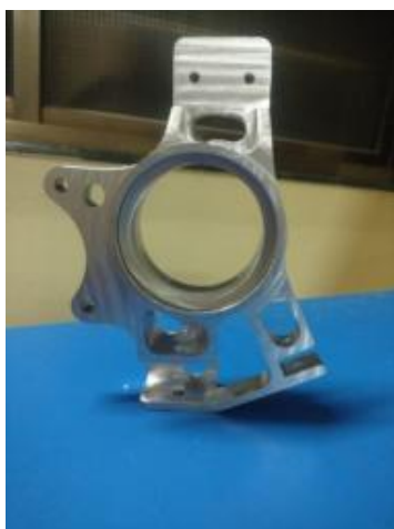
Fig 26 Finished front upright
