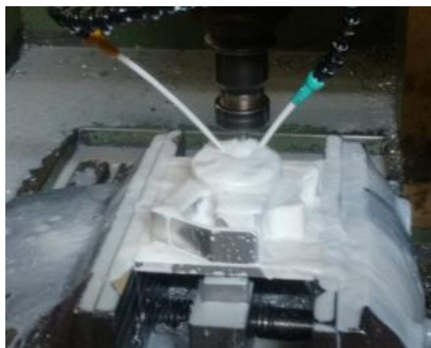
Fig 25 Machining of upright on a VMC machine
