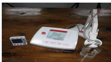
Fig.3: Measuring the Conductivity, salinity and TDS of magnetic water by conductivity
