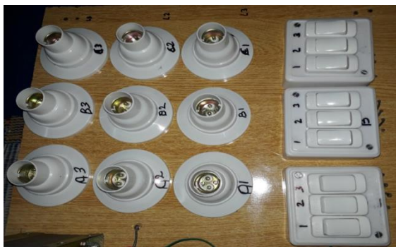
Figure 8 Implementation of Load Unit
