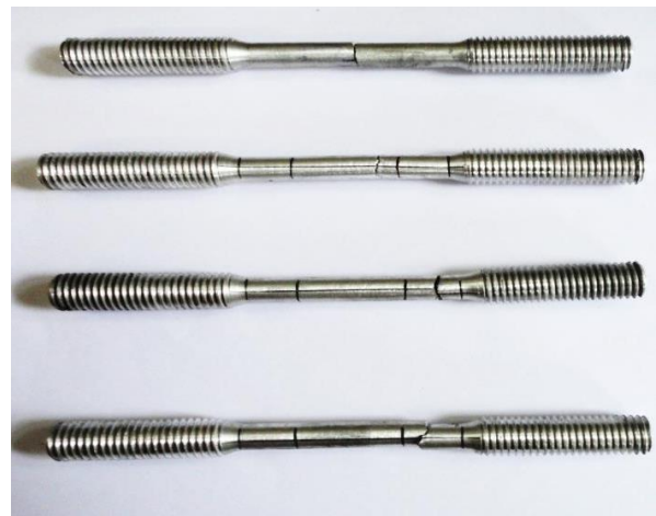
Fig.1 Tensile Specimens after Test
