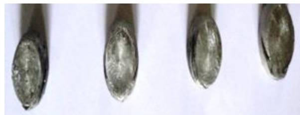
Fig.2 Compression Specimens after Test
