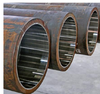
Figure 1 Image of cladded pipes
