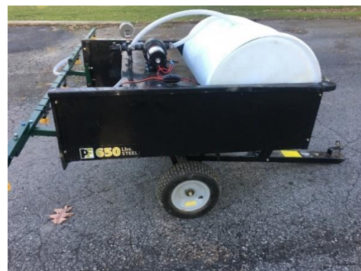
Fig. 2 Trailer with the 35-gallon tank, pump, hoses and feeding brackets
