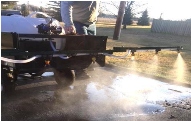
Fig. 7 Built unit in operation with all nozzles spraying as intended
