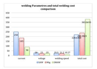
Fig. 15.Comparison of welding parameters and cost
