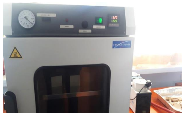
Fig.1 Thermal chamber used for the treatment
