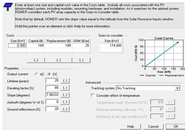
**Fig. 3.1: Solar PV model**
