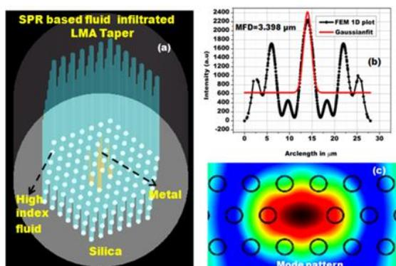
Fig. 4 Metal /high index fluid filled LMAPCF Taper
