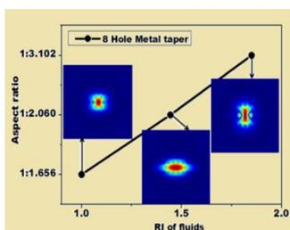
Fig.10 RI based tuning of aspect ratio for the same configuration of 8 metal filled and 8 tunable material infiltrated holes with beam profiles as inset
