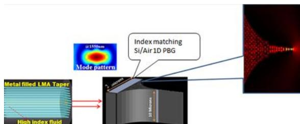
**Fig. 11** Proposed schematic of LMA PCF based SPR beam modifier for optical interconnection to silicon waveguides
