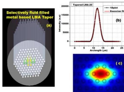
Fig. 5 Selective metal (yellow shade)/high index fluid RI (green shade) filling in LMA Taper (b) resulting elliptical mode pattern with fluid RI=1.4444 in LMA-Taper
