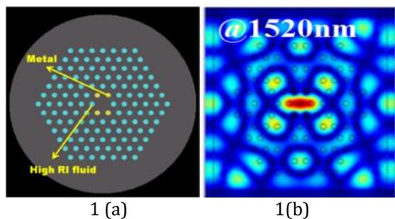
**Fig. 1(a)** Schematic of metal infiltrated LMA-20
