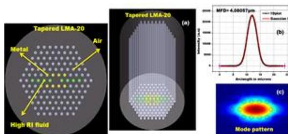
Fig. 7 Selective metal (yellow shade)/high index fluid (green shade) filling to generate LP01 mode pattern
