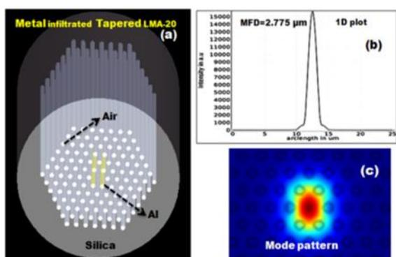
Fig. 3 Metal filled LMA-20 Taper with air holes
