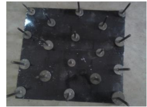
Fig.4. Staggered Rods as Roughness element on the absorber plate
