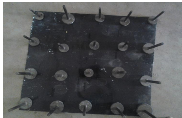
Fig.5. In Line Rods as Roughness element on the absorber plate
