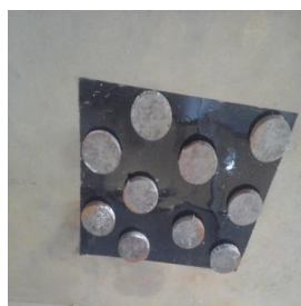
Fig.2. Cylindrical blocks as Roughness element on the absorber plate
