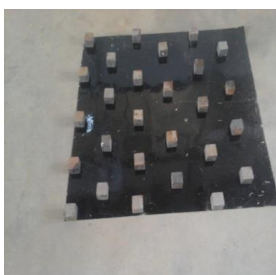
Fig.1. Cubical blocks as Roughness element on the absorber plate
