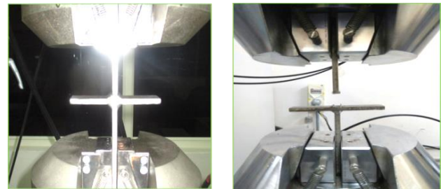
Fig 3. Specimen placed in Fatigue testing Machine
