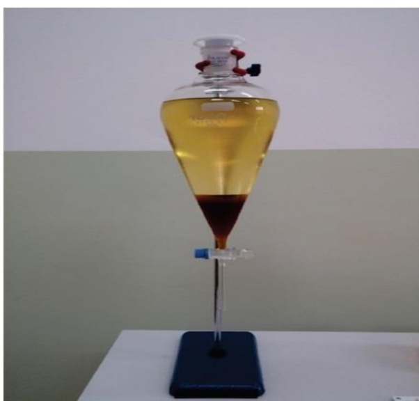
Figure 2.2 Solution after treatment left in standing funnel for settlement
