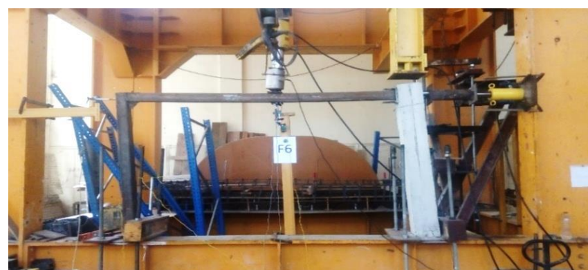
Fig 11: Failure Mode of Frame CS1
