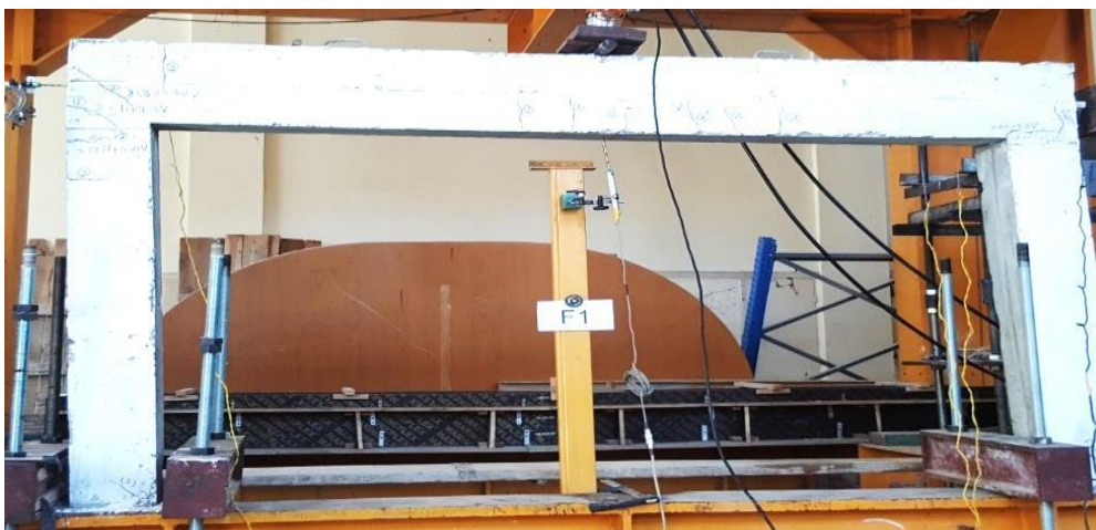
Fig 6: Failure Mode of Frame CC
