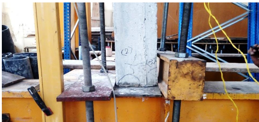
Fig 8: Failure Mode of Frame SC1
