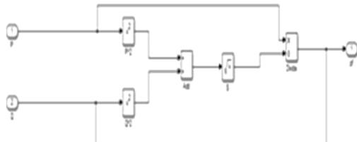
**Fig 7:** Power factor measure from active and reactive power
