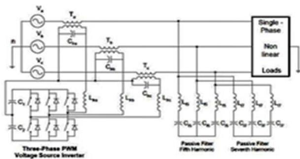
**Fig 4:** Series active power filter topology
