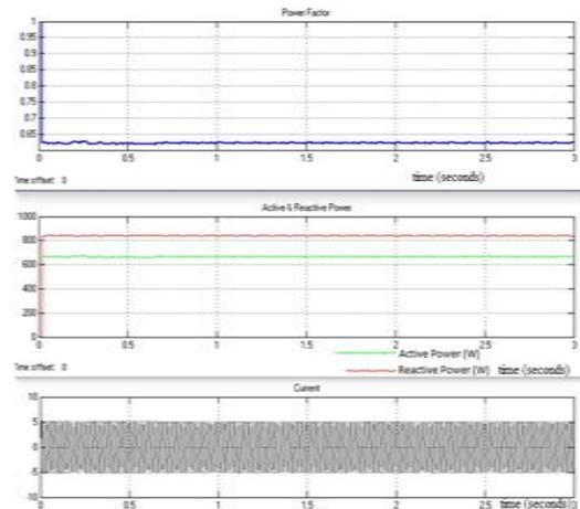
Fig 11: Scope output for power factor, Active & Reactive Power and Line Current for uncompensated system
