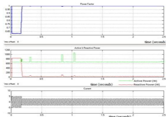
Fig 12: Scope output for power factor, Active & Reactive Power and Line Current for Compensated System
