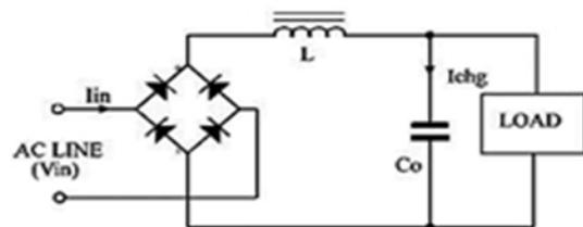
Fig 3: Block diagram of an Active Power Factor Correction circuit
