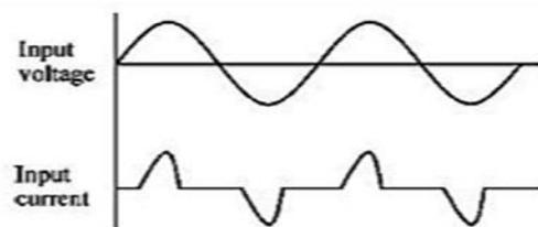
Fig 2: Input voltage and current waveform of a typical Passive Power Factor Correction circuit
