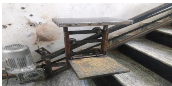
Fig.1 Actual testing Model of Chain drive Stairlift
