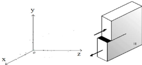
Figure 5: Mode-II, sliding mode of loading
