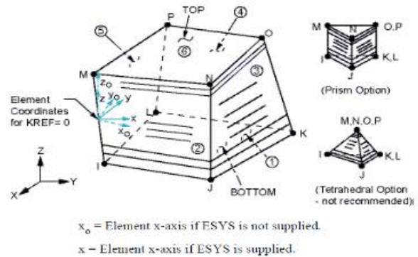
Figure 10: Solid46 DOF and element type
