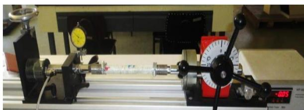
**Figure 3:** Torsion testing machine with specimen
