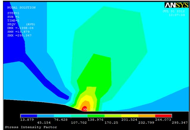
**Figure 16:** Von Misses stress of the cracked plate
