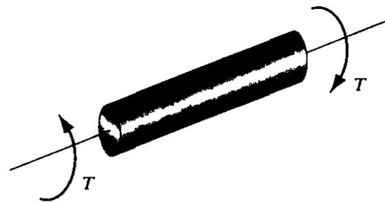
Figure 7: Transmission shaft subjected to torque
