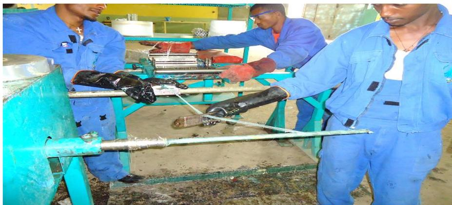
**Figure 2:** Manufacturing of the hollow transmission shaft
