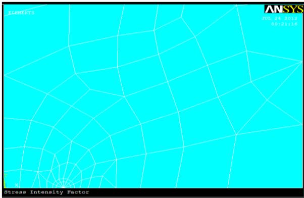
**Figure 13:** Meshed quarter part of plate with central crack
