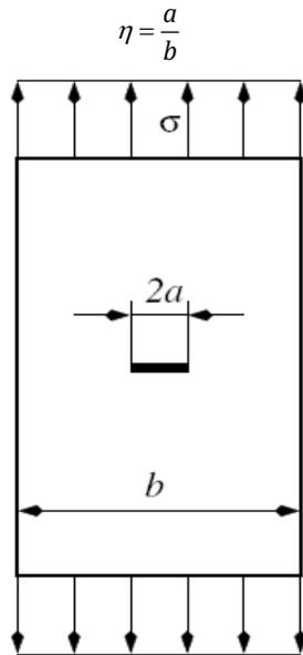
**Figure 8:** Through-thickness central crack
