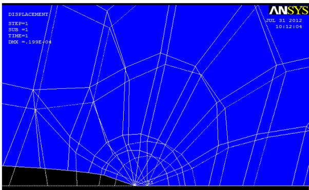
**Figure 14:** Deformation of the central symmetry crack
