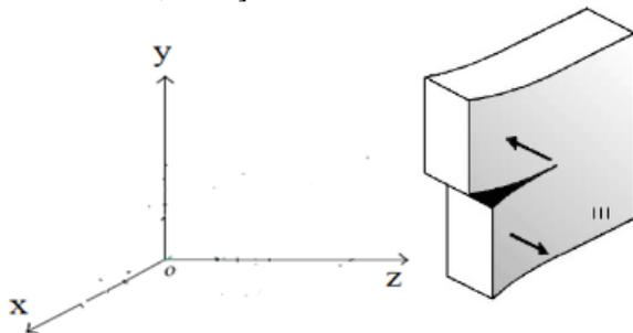
Figure 6: Mode-III, tearing mode of loading
