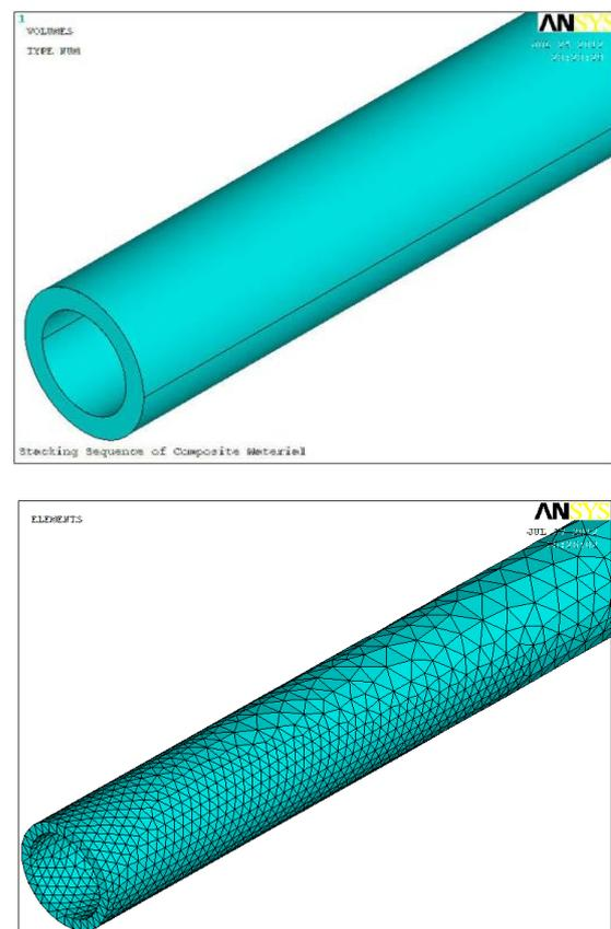
**Figure 12:** ANSYS model of a hollow transmission shaft (a) The zoomed 3D model (b) Zoomed Meshed model
