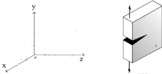
Figure 4: Mode-I, opening mode of loading
