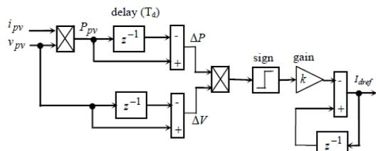
Fig.6: P&O algorithm implementation in Matlab/Simulink software
