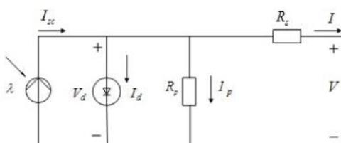
Fig.2 The equivalent circuit for a PV cell
