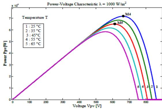
**Fig.4:** (P-V) characteristics of The PV Generator (NP=14 And NS=28) with constant radiation and varying temperature
