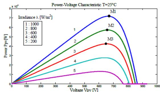
Fig.3: (P-V) characteristics of The PV Generator (NP=14 And NS=28) with constant temperature and varying radiation
