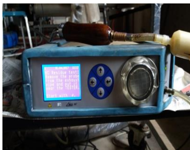
Fig 5.3 Exhaust gas analyzer
