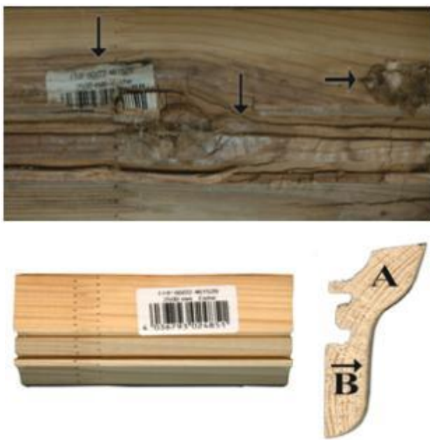
Picture 4: Attacked batten (up) and healthy batten (down)
