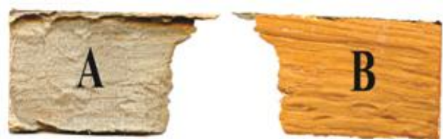
Picture 10: Thin layer of lacquered parquet flooring, A- inner, B-outer lacquered part
