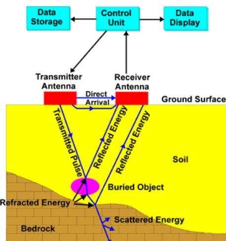
**Fig.1** GPR schematic, (from Environmental Protection Agency, Web site)
